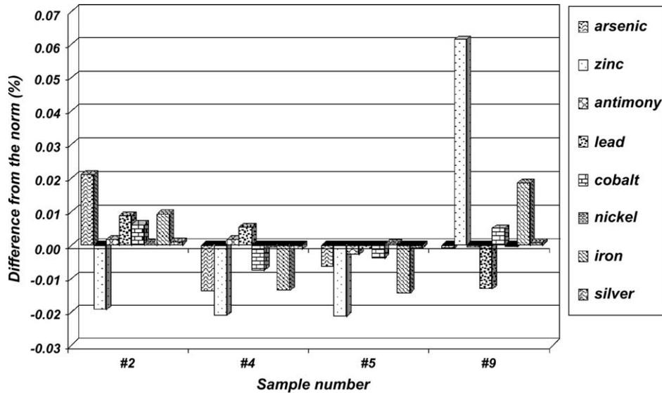
Fig. 10. Difference from the 'norm', analysis of trace elements in samples from the ram main cast.
