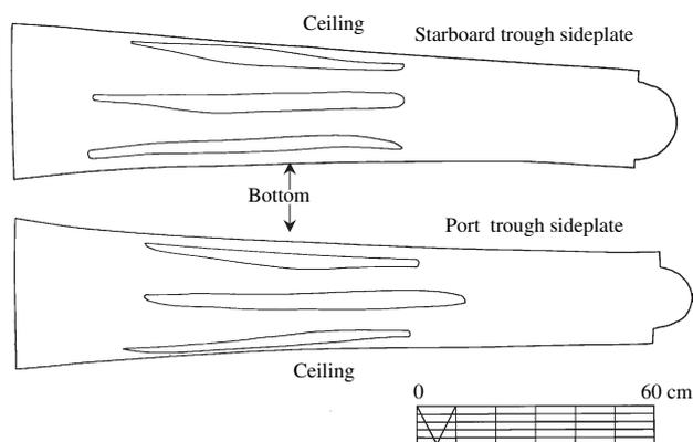
Fig. 6. The interior of the sideplates showing the dimensional variations in the plates and fin channels. (Drawing by A. Schreur and the author)
