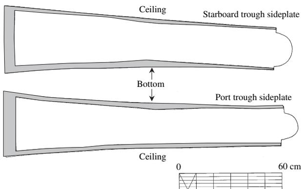
Fig. 8. Cowl ceiling and bottom plate wall thickness. The cross sections show the cowl ceilings and bottom plate wall thickness at their junction with the trough sideplates. (Drawing by A. Schreur and the author)
