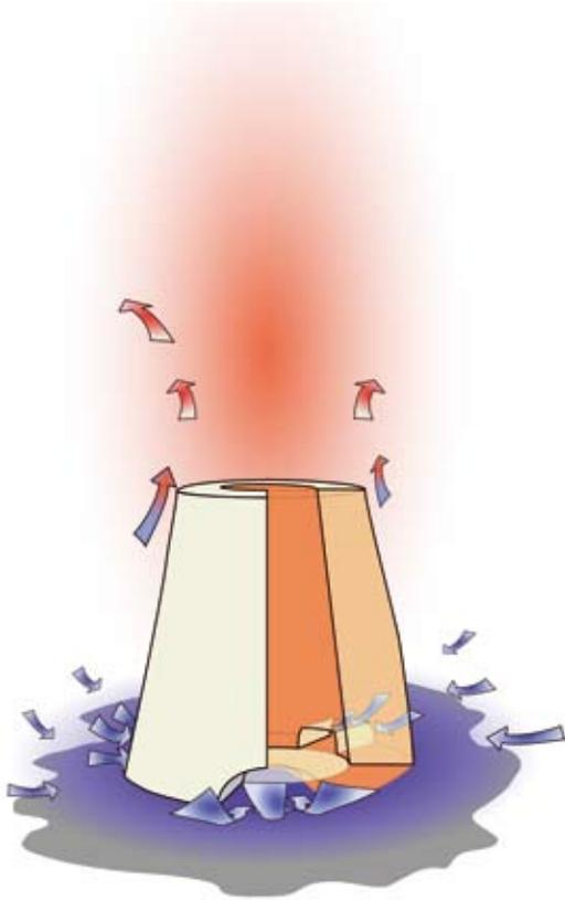
**Figure 6** Bernoulli's theorem: hot air rises, leaving a zone of lower pressure at air inlets. Atmospheric pressure compensates the lower pressure zone by pushing air into the inlets.
