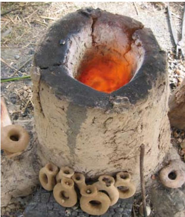
**Figure 9** Furnace after one week of continuous operation. Cracks may easily be repaired with fresh clay. Because of the conical shape, the furnace is unlikely to break apart.
