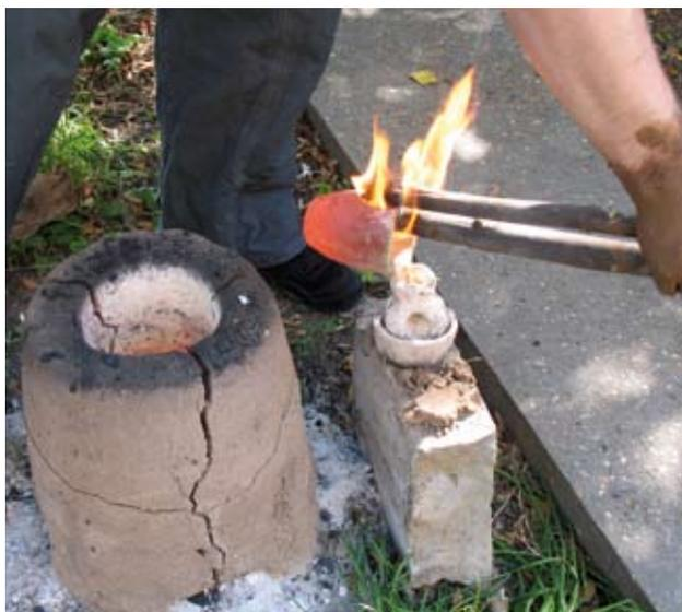
**Figure 5** Casting with wooden tongs.
