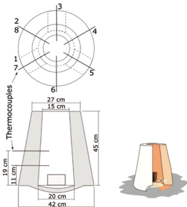
**Figure 1** Plan and side view of the experimental shaft furnace. The numbers 1–8 denominate the two principal sets of positions of the thermocouples; the side view shows the thermocouples’ elevation above ground.
