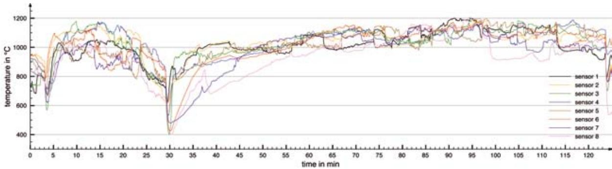
**Figure 2** Plot 1: an episode with the shaft fully charged with charcoal. Note that the y-axis starts only at 300 °C.
