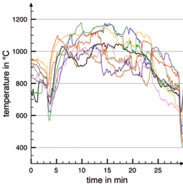
**Figure 3** Plot 2: shaft half-filled with charcoal. Note that the y-axis only starts at 300 °C.
