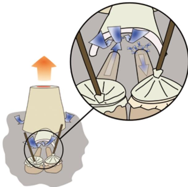
**Figure 7** The hydrodynamic paradox: objects bordering streaming fluids are pulled towards them and not pushed away.
