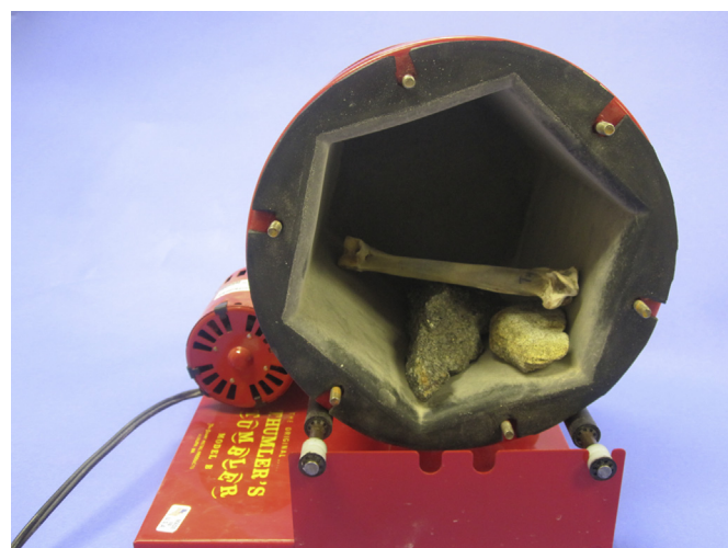
Fig. 2. The rubber-lined hexagonal rock tumbler used for the tumbling experiment. It rotates at 40 rpm and has a 15 lb. capacity (approximately 5 L in volume). It was sealed shut with a rubber-lined lid during the experiments.
