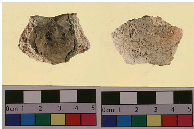
Fig. 2. One of the fragments of crucible H76-S66, showing the slagged interior surface (left) and the finished rim shape (top side). Although not shown in black-and-white imagery, the non-slagged side of this fragment shows remnants of the red ochre used to paint the exterior surface before the addition of chaffy, non-refractory technical ceramic layers.
