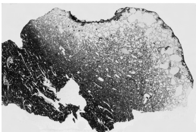
Figure 2: Thin section through a crucible fragment from Wetzikon-Robenhausen (Inventory number 32981 of the Swiss Landesmuseum). Note the thick body, and the very limited vitrification layer near the rim of the vessel, top and right. Width of image ca. 3 cm.
