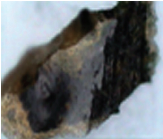
Figure 2 A photomicrograph of the yellow transparent material that was found covering the Ibis (1616). This coating material is strongly adhered to the black patina. Magnification \times 100 .
