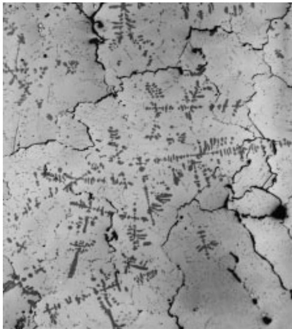
Figure 18. Microstructure of ingot 3391: large grains of primary  $\gamma$ - $\text{Cu}_3\text{As}$  alloy (pale grey) and  $\text{Cu}_2\text{S}$  matte dendrites (dark grey). Magnification 100. As polished.
