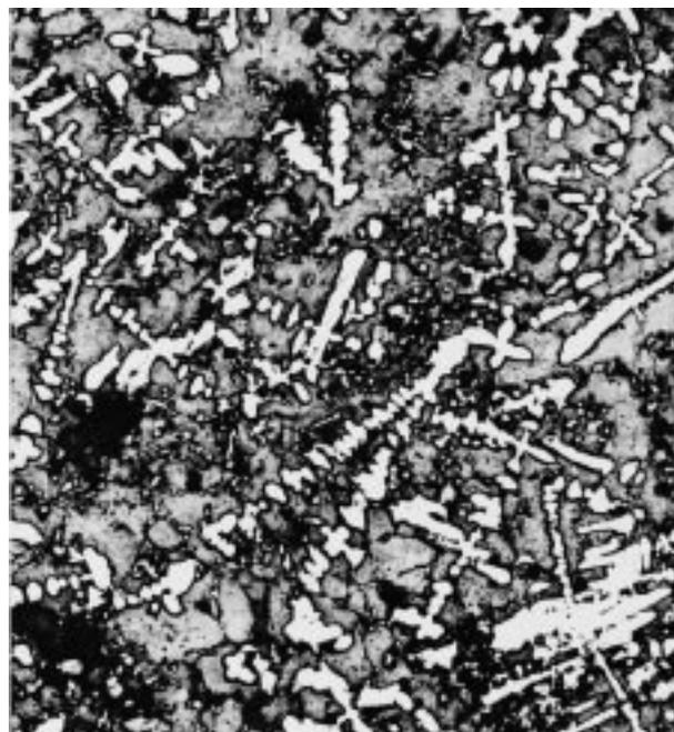
Figure 7. Microstructure of crust 3389: dendrites of  $\text{Cu}_2\text{S}$  matte (white) in an interdendritic groundmass of nantokite and calcium sulfite sulphate. Magnification 100. As polished.
