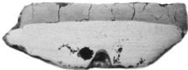
Figure 10. Section through matte layer and alloy ingot of furnace product 3396. Note thin layer of copper metal at the interface between matte and alloy. As polished.
