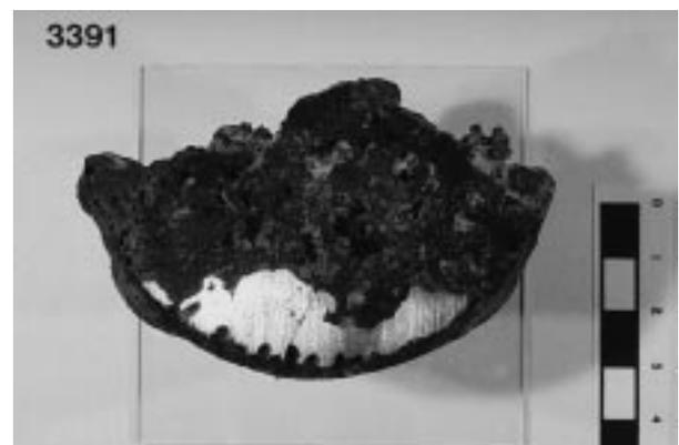
Figure 17. Section through crucible cosmelted product 3391. The highly reflecting alloy collected and solidified as an ingot at the bottom of the hemispherical mould.
